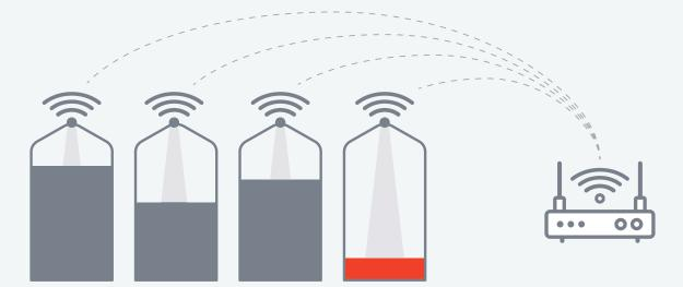
The Feedlink silo and tank monitoring radar sensor is wireless and solar-powered, removing the added expense of hardwiring by an electrician. Feedlink takes measurements every 30 minutes to provide reliable inventory information at your fingertips via your smartphone or PC.
