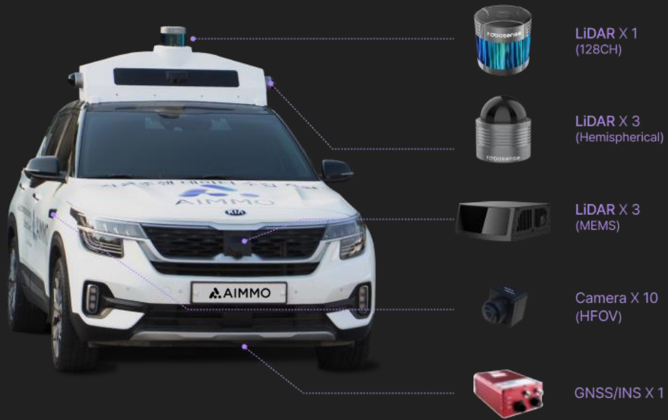
AIMMO's data collection Vehicle for autonomous driving
