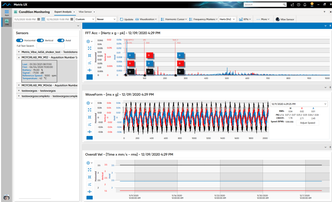
List of sensors (left) and Expert analysis, including Frequency markers
