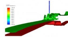
Slamming forces from breaking wave and actual bathymetry. The simulations were performed with ANSYS Cloud HPC resources.
