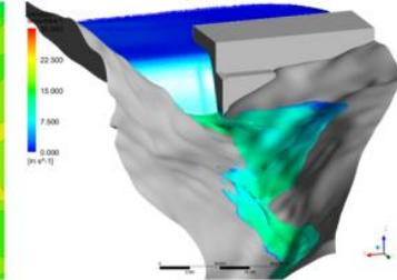
Flow simulations of waterway for design of new dam
