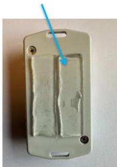
2. We can also use a small screw to screw up the devices in the ceiling or other required places. The devices have both side screwing holes.
