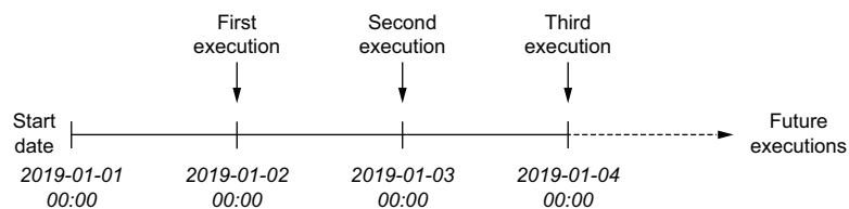
Figure 3.1 Schedule intervals for a daily scheduled DAG with a specified start date (2019-01-01). Arrows indicate the time point at which a DAG is executed. Without a specified end date, the DAG will keep being executed every day until the DAG is switched off.
