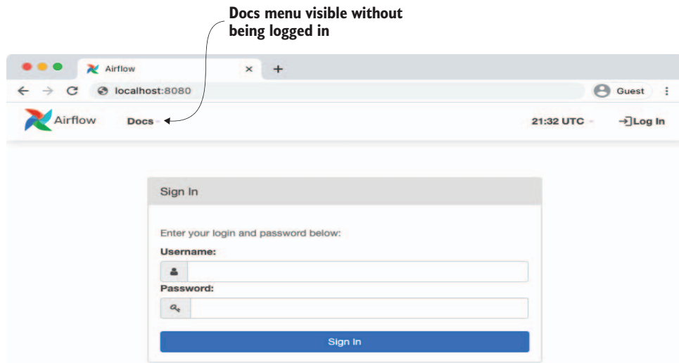
Figure 13.6 Granting permissions to the public role makes components of the UI available to everybody.
