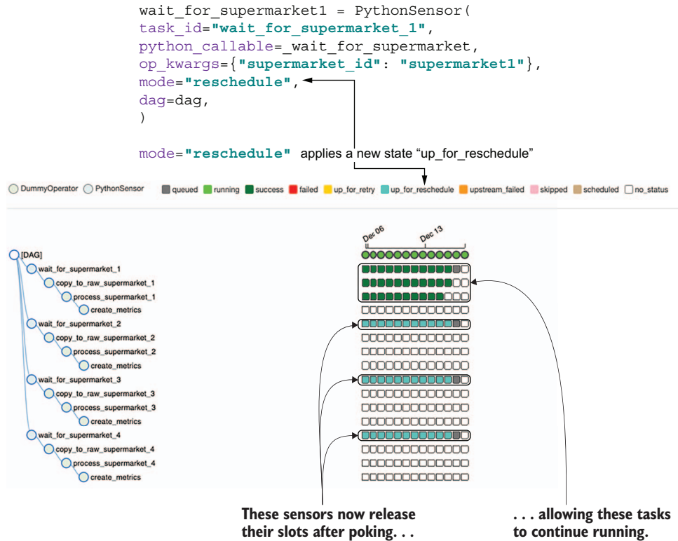
Figure 6.9 Sensors with mode="reschedule" release their slot after poking, allowing other tasks to run.
