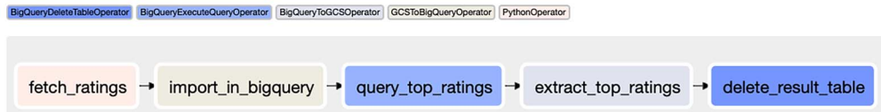
Figure 18.17 The complete DAG for downloading ratings and uploading and processing using GCP BigQuery
