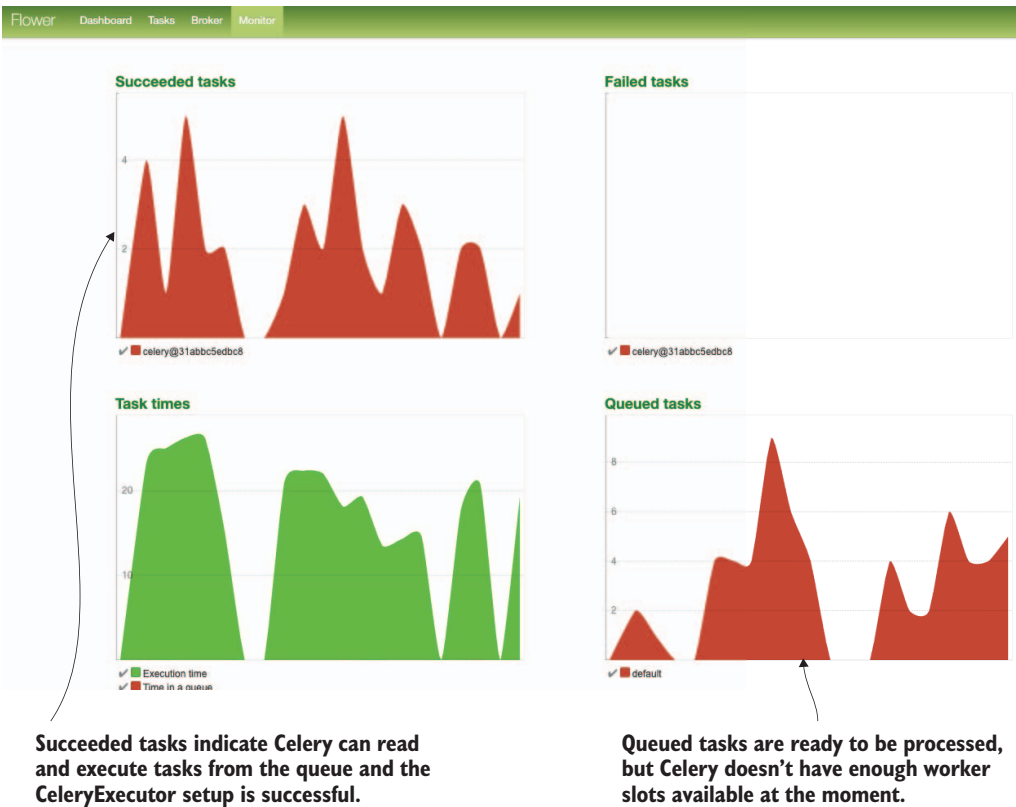
Figure 12.9 The monitoring tab of Flower shows graphs to understand the performance of the Celery system.
