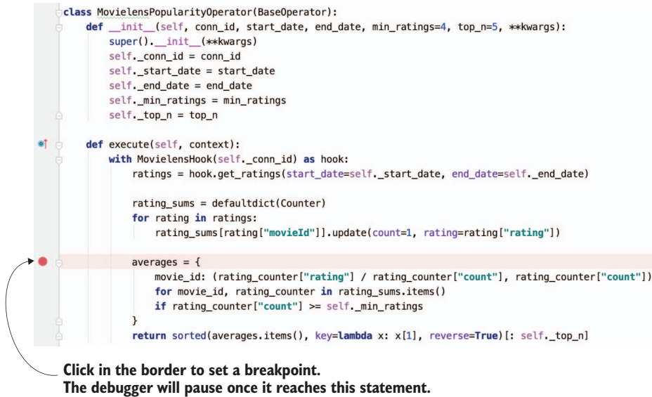
Figure 9.12 Setting a breakpoint in an IDE. This screenshot was taken in PyCharm, but any IDE allows you to set breakpoints and debug.
