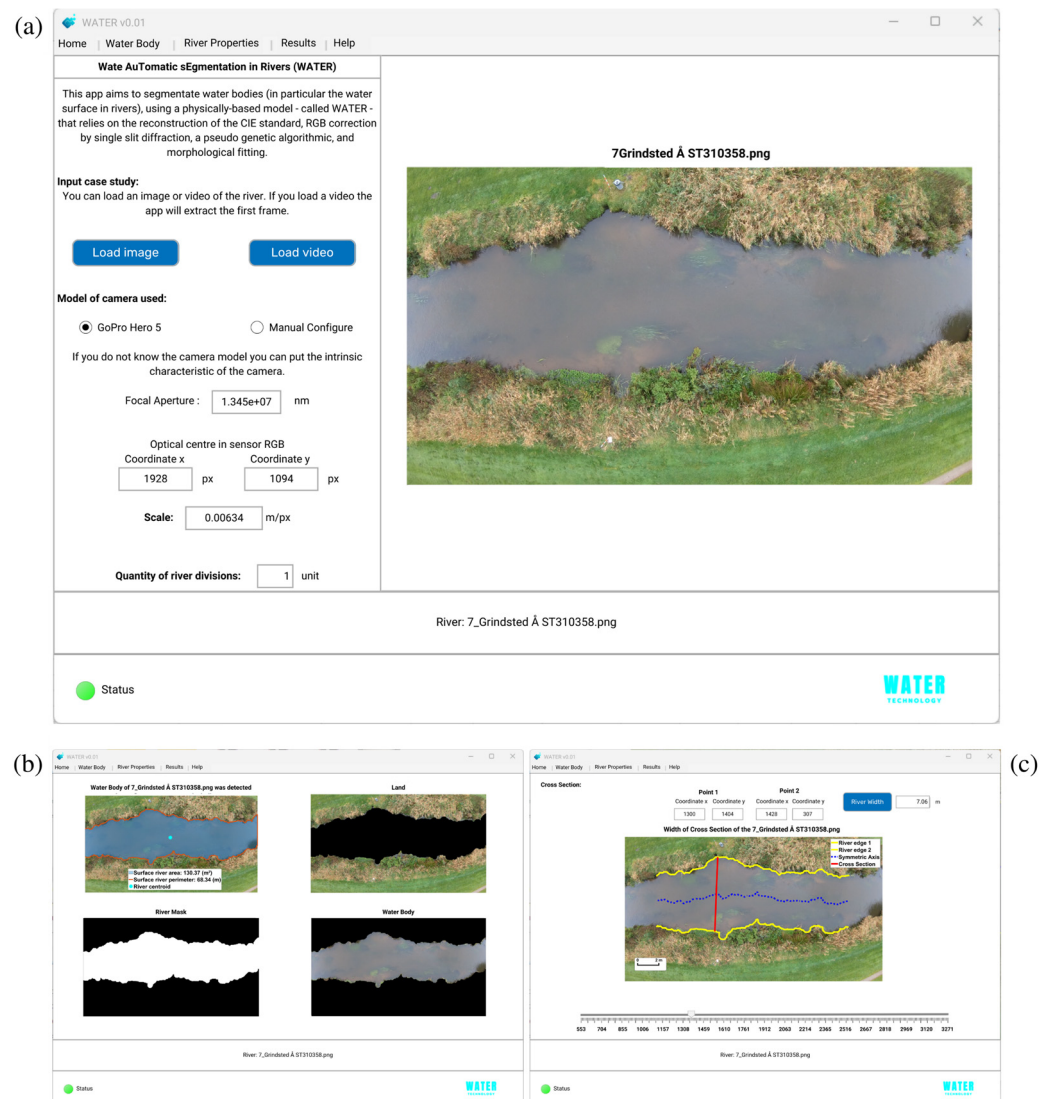
Figure 11. WATER software GUI with Grindsted case study (only for illustrative purposes, ID 6 in Supplementary Material E). (a) Home tab; (b) Results (river mask); (c) Results (symmetry axis and river width).
