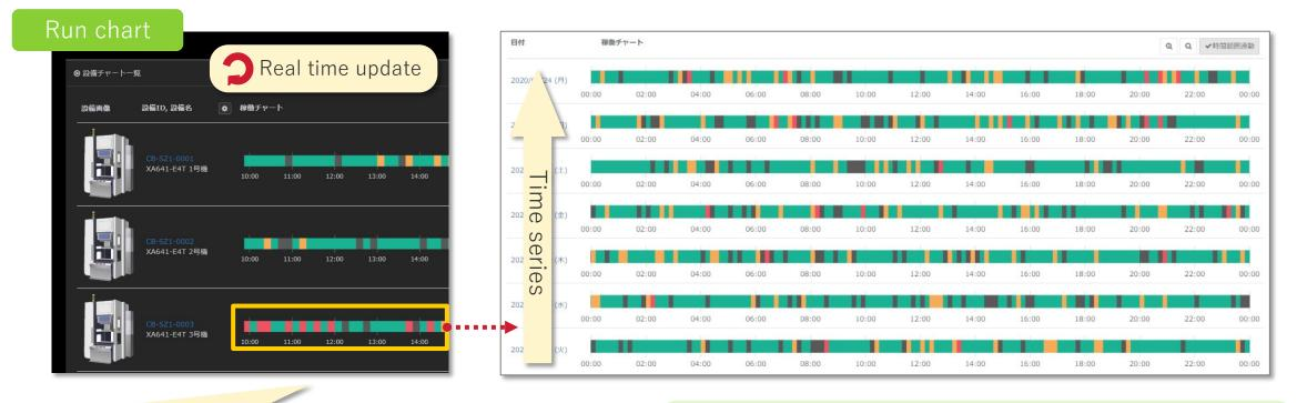
Color-coded display of device status such as shutdown, idle, and power off.
