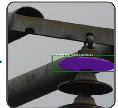
**Conclusion:** The integration of Azure Custom Vision Model and Segment Anything Model in the development of a corroded insulator shells detection system exhibits high precision and recall. This integrated model demonstrates promising potential in detecting and segmenting corroded parts at an early stage, thereby enabling predictive maintenance measures.
