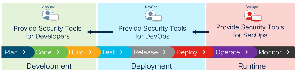
Figure 2: Shifting Security Left in the CI/CD Cycle
