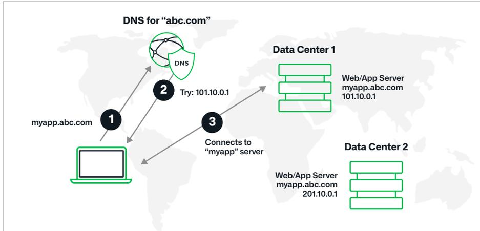
Figure 3: DTC provisioning showing 1) app deployment initiation, 2) company DNS connection, and 3) myapp server provisioning in distributed data centers.
