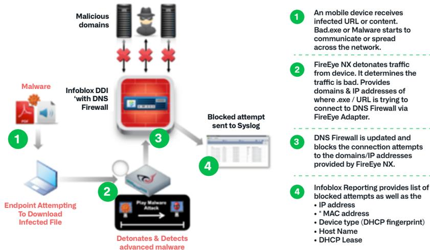
Figure 2: How DNS Firewall works to block malicious connection attempts.
