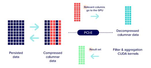
Flgure 2: Data flow from disc storage, through main memory RAM to GPU RAM.
