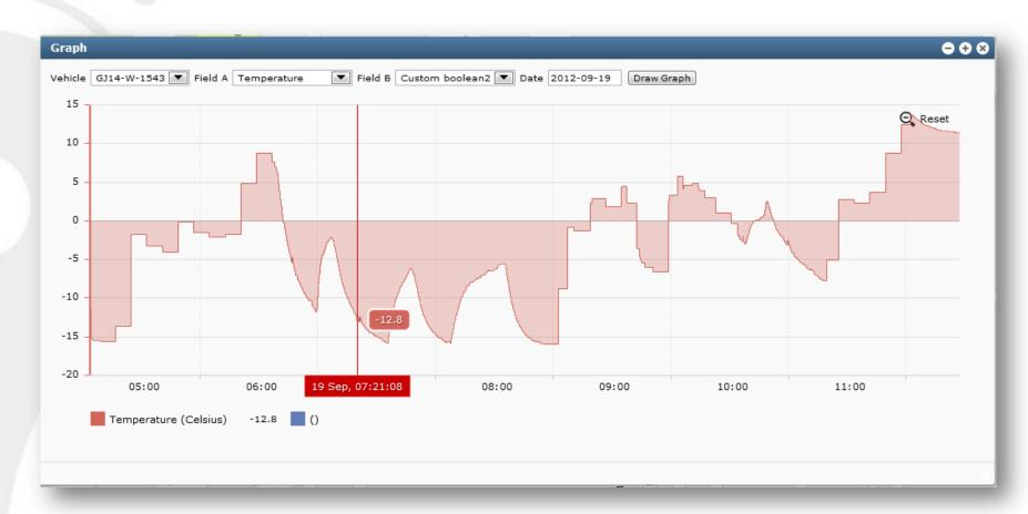
Temperature Graph of cargo provides you with detailed point-to-point temperature history of the Cargo. This can be used in Quality Control and ensuring cargo movers are pro-active to quality.
