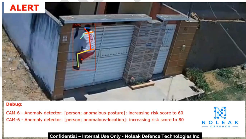
Figure 3 -Example of a residential intrusion detected by Noleak Agatha
