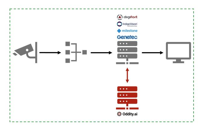
The systems work with both analog and digital cameras. No new cameras need to be installed. The server is plug-and-play, so it can be removed from the infrastructure at any time, without disruption. Alarms are sent back the way the user wants.
