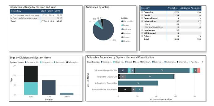
Cognitive Integrity Management<sup>™</sup> (CIM) is a born-in-the-cloud Software-as-a-service "SaaS" solution that manages the compliance and integrity of oil and gas assets. CIM is a fully integrated enterprise-level solution in the highly secure Microsoft cloud that uses advanced data science and machine learning to assist pipeline operators in managing the integrity and risk of their assets through the integration, alignment, analysis, and reporting of assessment data and information.
