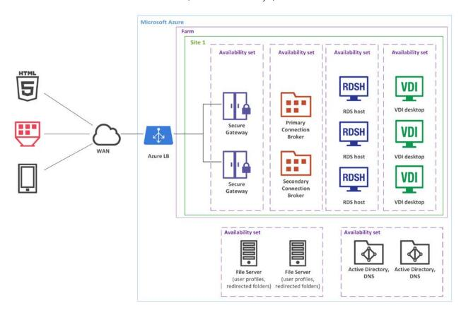
You can also use Azure as a SAML IdP provider and as cloud computing platform for VDI/RDS resource hosts to deliver applications and desktops.
