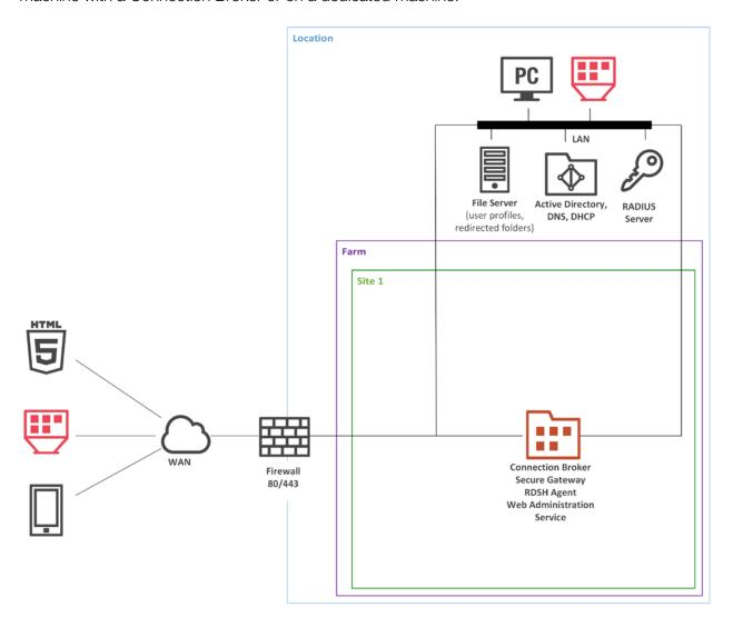
In this scenario, all components, including RAS Web Administration Service, are installed on a single RD Session Host. This configuration is only recommended for proof-of-concept and small environments.
