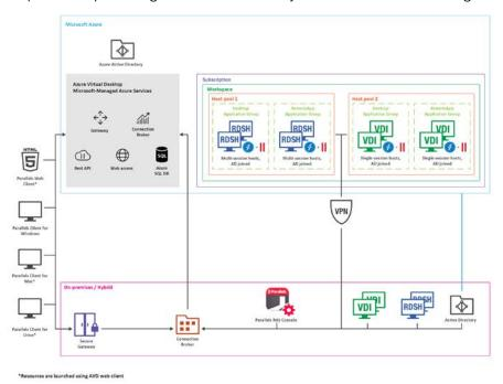
As highlighted earlier, the complete Parallels RAS environment can also reside on Microsoft Azure for a full cloud deployment with Azure Virtual Desktop.
