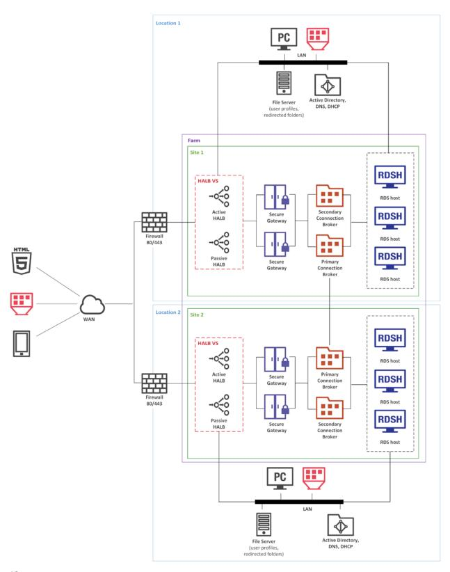
Each site consists of at least a RAS Connection Broker, RAS Secure Gateway (or multiple Secure Gateways), and agents installed on RD Session Host or VDI servers, or Windows PCs.
