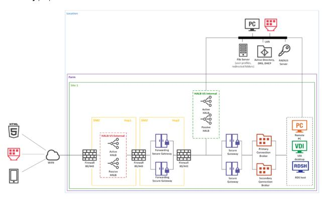
Parallels recommends using Forwarding RAS Secure Gateways in double hop DMZ deployments only.
