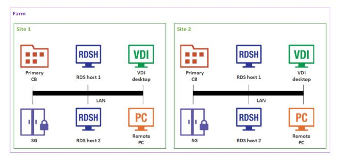
Adding more RAS Connection Brokers and RAS Secure Gateways adds redundancy to the system. HALB Virtual Server (VS) is a virtual representation of the HALB appliances (optional component), which can be added to load balance application traffic.
