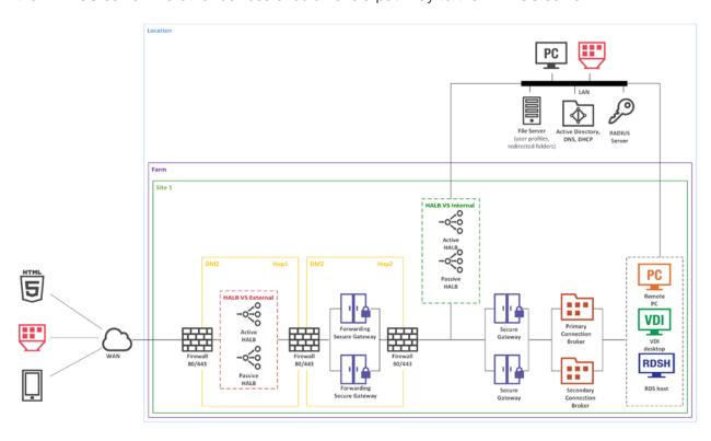
In a configuration of this type, the second-level authentication via a RADIUS server is performed first. If the authentication procedure is successful, the next authentication takes place at the Active Directory level using either the username and password or a smart card.
