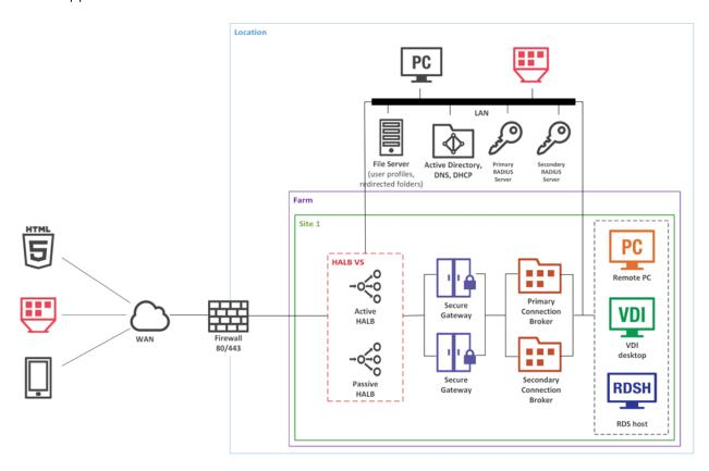
Please note that the diagram above includes an optional secondary RADIUS server which can be used as active/active or active/passive to provide high availability.
