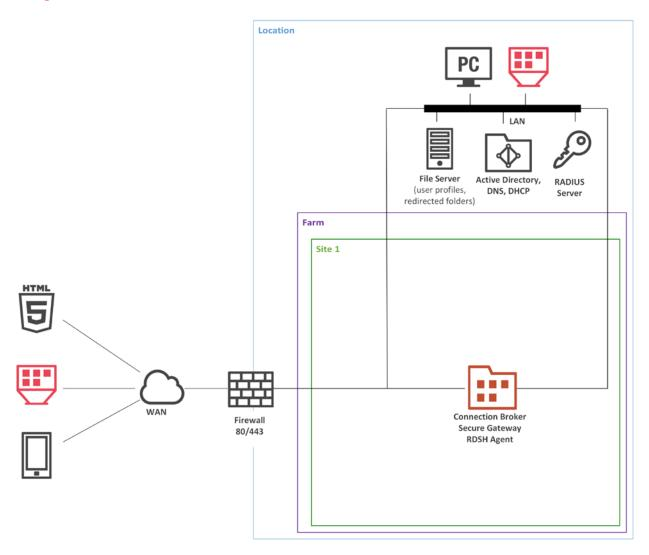
This scenario uses a single RD Session Host for publishing applications and desktops. SSL and User Portal are enabled by default with a self-signed server certificate. The server certificate should be trusted by client devices. Enterprise certificate or third-party trusted Certificate Authority can be used for external access (for details, please see the **SSL Certificates** section (p. 69)).
