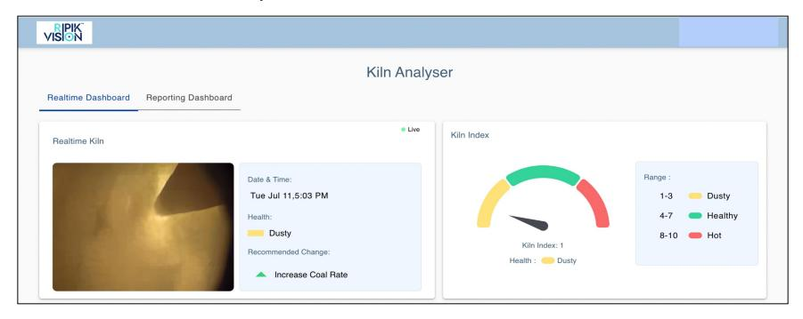
The Image shows the latest kiln image along with the health of the kiln and kiln index
