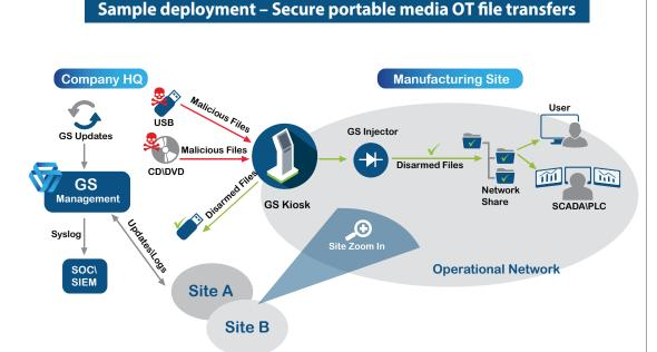
Centrally managed, geographically distributed Kiosks at multiple sites. Files are copied from portable media and multi-scanned/disarmed to trusted media, or delivered securely using a data diode (GateScanner<sup>®</sup> Injector).
