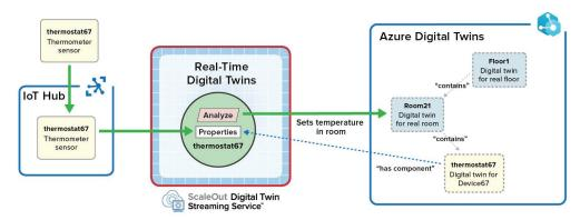
Note that the ScaleOut Digital Twins Streaming Service takes responsibility for ingesting messages from Azure IoT Hub and for invoking analytics code for the data source's incoming messages. Multiple, pipelined connections with Azure IoT Hub ensure high throughput. Also note that the two serverless functions and use of Event Grid have been eliminated since the in-memory method handles both message processing and updates to the parent object (Room 21).
