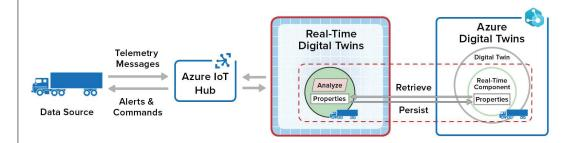
Each truck has a corresponding Azure digital twin which tracks its properties including a subset of real-time properties held in a component of each instance. When telemetry messages flow in to Azure IoT Hub, they are processed and analyzed by ScaleOut's in-memory computing platform using a real-time digital twin that holds a truck's real-time properties in memory for fast access and a message-processing method that analyzes telemetry changes, updates properties, and signals alerts when needed.
