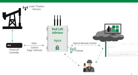
The overall effectiveness of rod lift operations can be limited by various factors that may result in deferred production or other operational efficiencies. Furthermore, rod lift wells have often been managed reactively, resulting in missed opportunities to maximize production. While increased access to rich data adds value, there is no direct impact on the effort required to take proactive measures to fully optimize rod lift operations.
