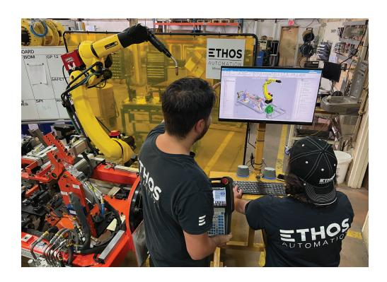
"We can do a lot of the debugging by using Process Simulate. We can actually see if there are going to be any anticipated issues and zone the robots out between each other based on these issues."
