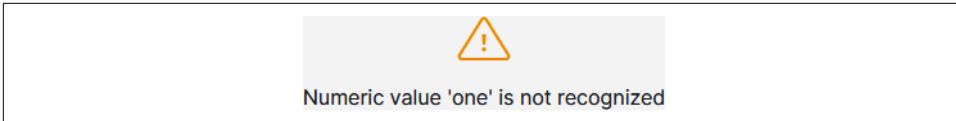
Figure 4-8. The error message that is received when attempting to insert two different data types into a VARCHAR column in one multirow INSERT statement
