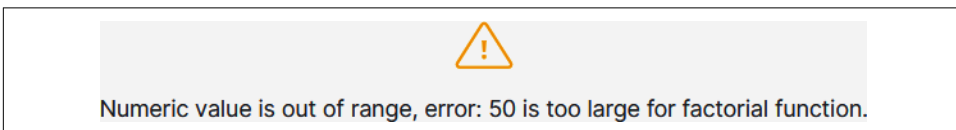
Figure 3-26. An error message is received because the number 50 is greater than what can be used with the FACTORIAL function
