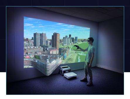
The Holo-Wall Go creates a 2x3.5m screen which visualizes 3D information. While being similar to the Holo-Wall this portable variant can be packed in two rugged cases for easy transport.
