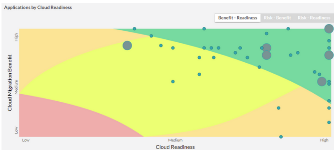
Cloud readiness scoring of the entire application portfolio compared to potential benefits of moving application to the cloud. This report helps identifying quick wins and early migration candidates
