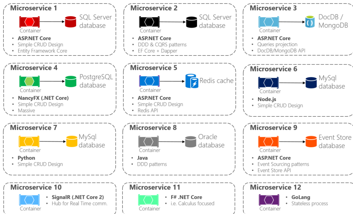
Figure 6-3. Multi-architectural patterns and the polyglot microservices world
