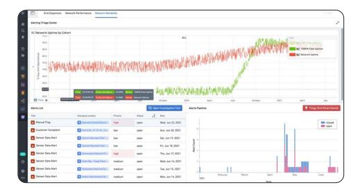
Users can manage large networks of chargers at scale with operational tools built right from chargers' IOT sensor data. They can monitor and improve the performance of individual chargers by tracking uptime via OCPP sensor data and reveal the historical performance of each owned or publicly available charging station, its daily utilization, and electricity costs where data is available.
